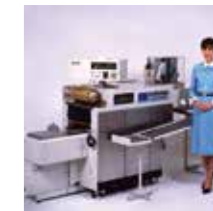
World's first integrated weighing, wrapping and labeling machine
